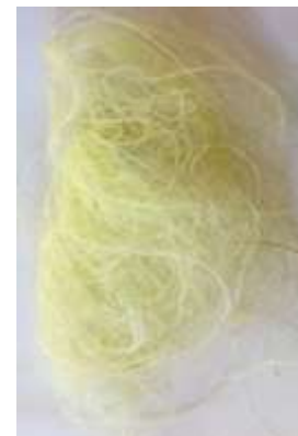
Figure 8 Habarala ( Alocasia macrorrhizos (L.) G.Don) fibre after chemical treatment.
