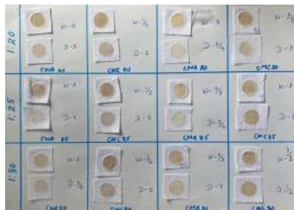
Fig. 1. Staining of the dry (D) and wet (W) rubbing cloths for all twelve treatments. Columns, left to right: aqueous extraction with alum (CWA) and with copper sulphate (CWC), then methanolic extraction with alum (CMA) and with copper sulphate (CMC). Rows are the dyebath liquor ratios 1:20, 1:25 and 1:30. Labels on the photograph carry a leading C for cinnamon, so CWA20 corresponds to WA20 in the text.
