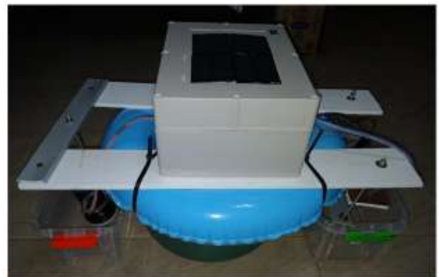
Fig. 2. Fully assembled buoy prototype with integrated sensing, communication, power and ultrasonication subsystems.
