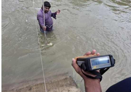
Fig. 4. Current-meter discharge measurement in the canal.
