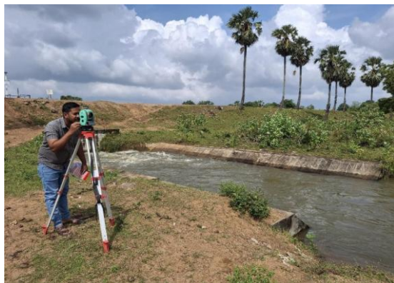
Fig. 3. Total Station surveying along the Kaddumurivu main canal.
