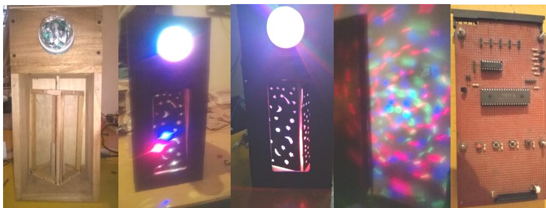
Figure 7: Implementation of Soothing system (Mechanical and Electronic circuit)
