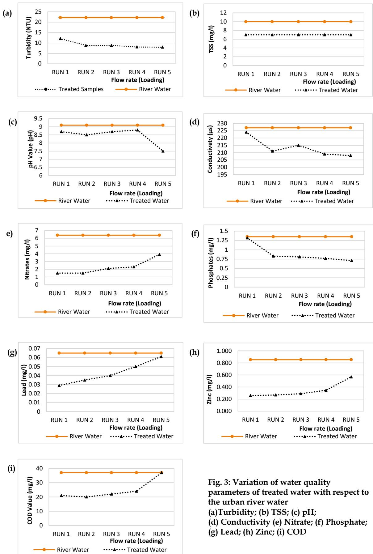
**Fig. 3: Variation of water quality parameters of treated water with respect to the urban river water**
