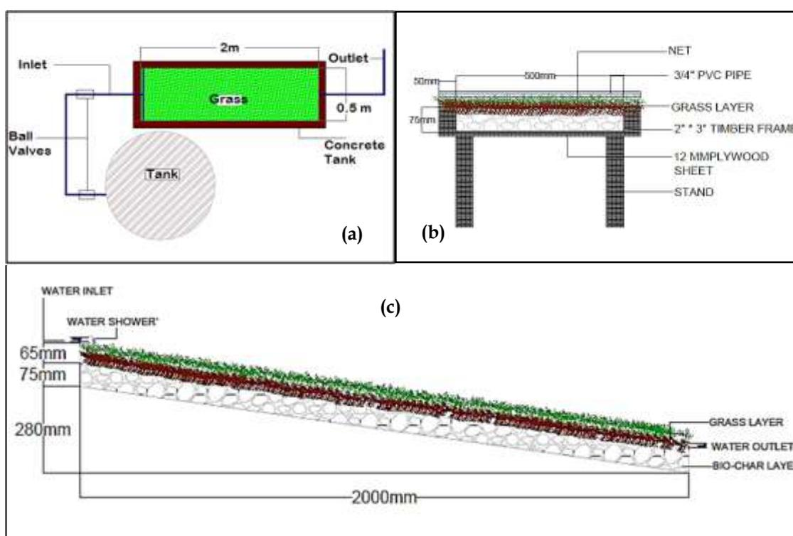
**Fig. 1: Details of biochar embedded bio geo filter experimental setup**
