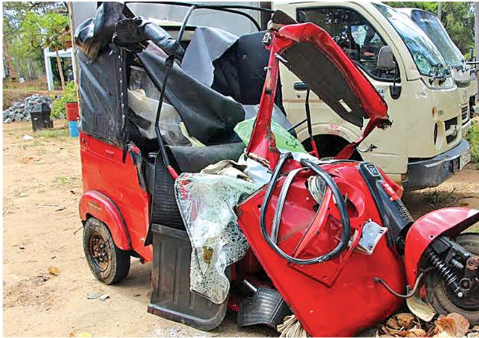
Fig. 11. An accident with the front face intrusion killing the driver. [Daily News 2016]
