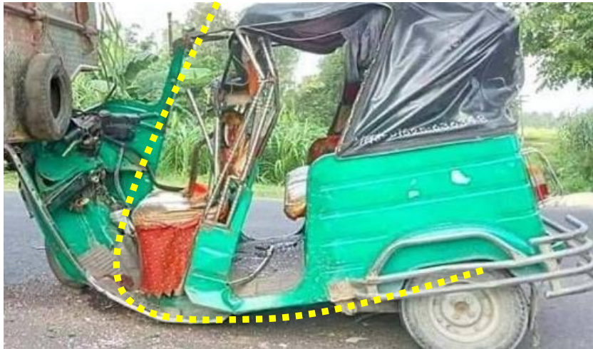
Fig.1. Head-on collision of a conventional three wheeler against a rigid barrier (Numan 2022).
