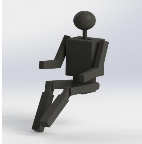
Fig. 5. Custom Human Hybrid III 50th Male Model
