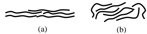
Figure 3: Model illustrating PANICAS polymer chain arrangement in a (a) thin film (b) thick film
