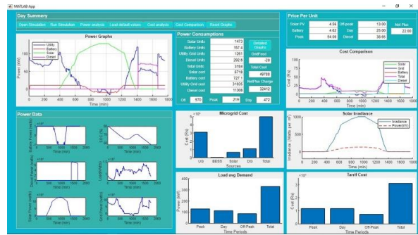
Figure.6. Day summary of the microgrid that shows power dispatch, the energy cost of the sources, power during peak, off-peak, and day time, and tariff structure
