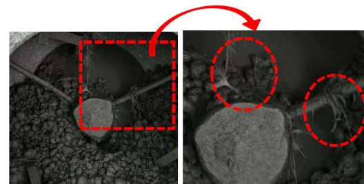
Figure 1. The mixer blade was encircled by long (50 mm) fibers that gathered into clusters
