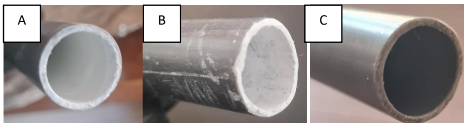
Figure 11: PVC pipes: (A) painted, (B) nanocoated with synthesized ZnO and TiO 2 nanoparticles, (C) uncoated.
