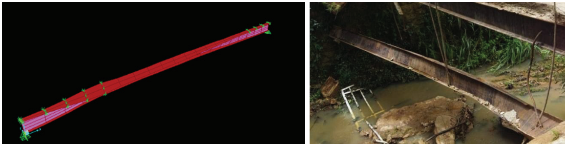
Fig. 11. Deformed shape of beam at end of the buckling analysis in SAP2000
