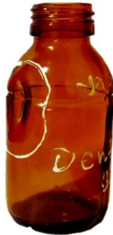
Fig. 1. Defective Container (Dented Body)
