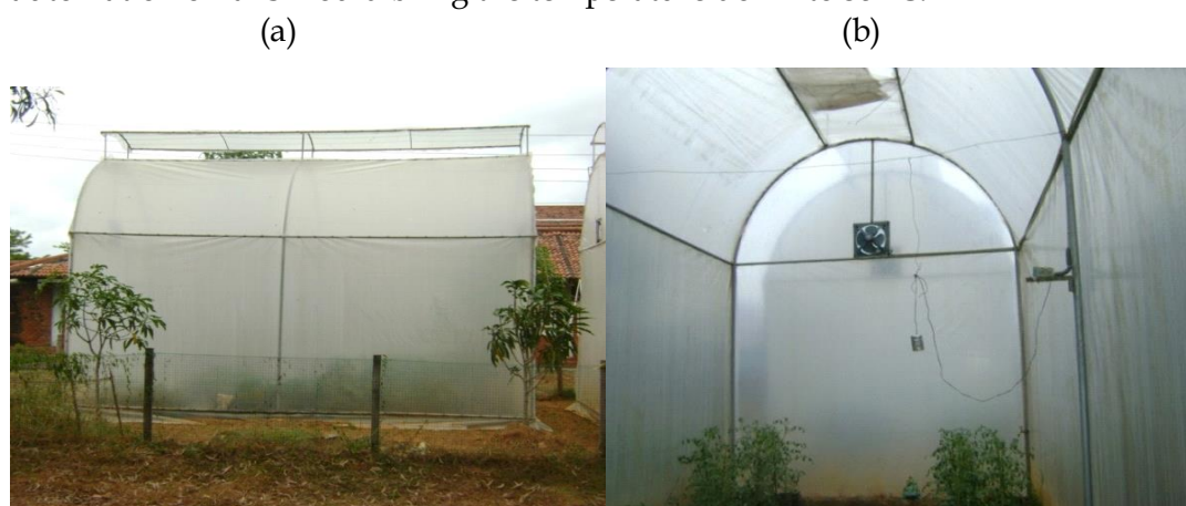
Fig. 2. (a) The External and (b) Internal View of the Polytunnel in which the Plants were maintained at a Maximum Temperature of 35 °C
