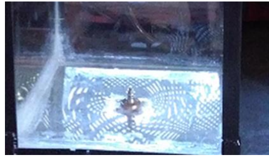
Fig. 4. A closer look of the nozzle assembly fixed to the bottom of the tank
