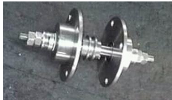
Fig. 6. Fabricated nozzle and pulley arrangement
