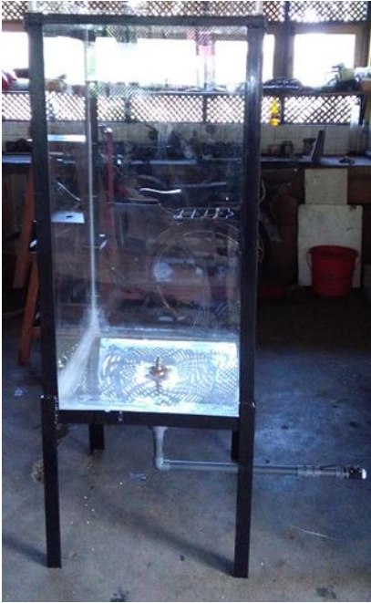
Fig. 3. The tank with transparent Perspex walls
