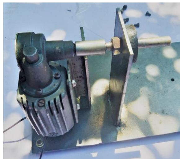
Fig. 9. DC geared motor used for rotating the coconut
