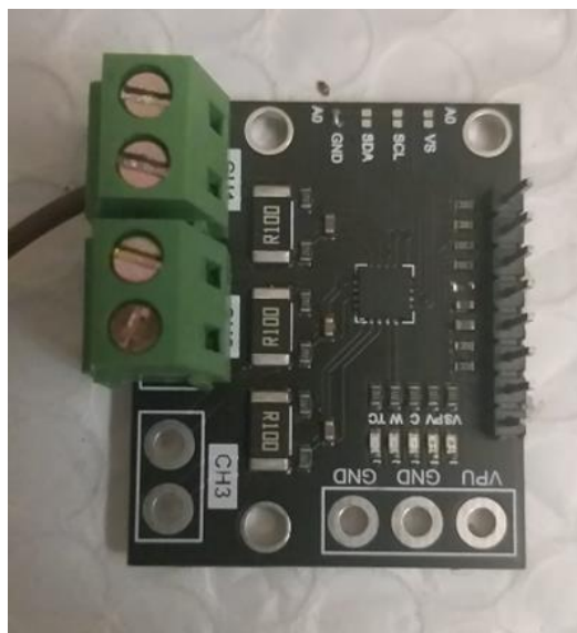
Fig. 10. INA3221 as Current Sensor
