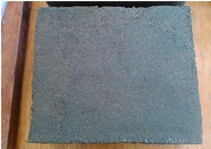
Fig. 16 1: 6 plastering coat - 30% bottom ash replaced
