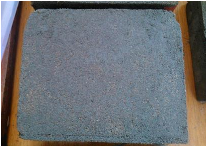
Fig. 15 1: 6 plastering coat - Control mix
