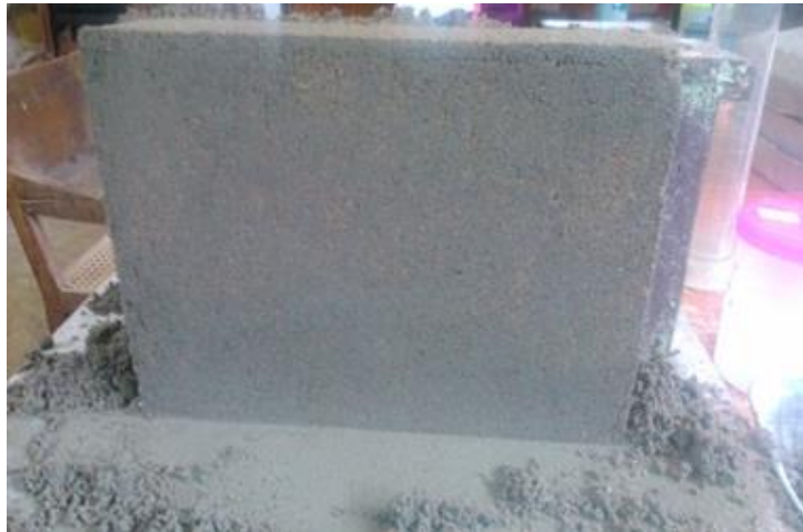
Fig. 14 1:5 plastering coat - 30% bottom ash replaced
