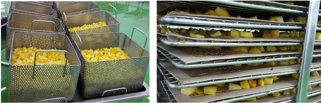
a. Chips at water removing stage b. Wet chips on racks before send to dryer
